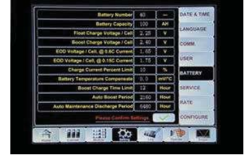
Permit the first commissioning without using of external tools. The password protects against accidental access and dangerous settings.
