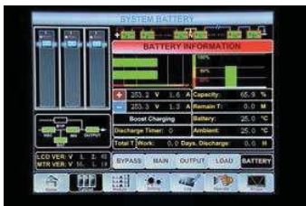
The discharging timer and total battery working time permit to make a precise analysis of the health of the batteries and to organize preventive battery maintenance scheduling
