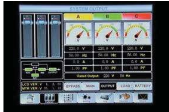
Recordable working status: voltage, warning, alarms and power of bypass input and output.
